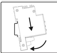
Modules must be installed within a suitable surface mount enclosure with integral DIN rail. Installation must be carried out by a qualified electrician in accordance with National Wiring Regulations and other applicable regulations. Compliance to EC EMC and Low Voltage Directives may be invalidated if not used or installed according to the published specification.
