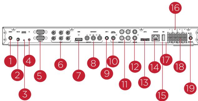
**1** ZigBee. The antenna for the ZigBee radio.
