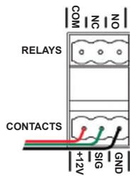
Figure 5. Contact for Dry Contact (e.g., Door Contact Sensor)
