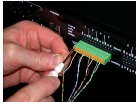
**EXAMPLE:** If you add a motion sensor (see Figure 5), connect its wires to the following Contact openings:
