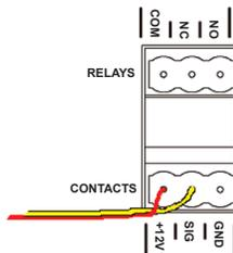
Figure 6. Contact for Self-Powered Voltage Source Device
