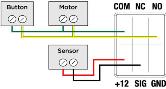
Figure 9. Connecting a dual-relay device (blinds)
