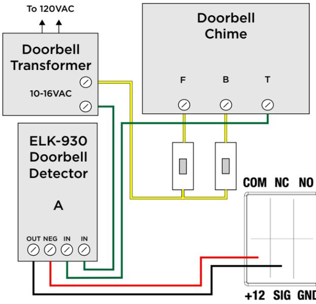
Connecting the relay ports
