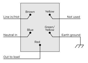
Figure 3. Single device location, without neutral connection
