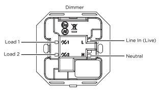
Figure 3: Single device location, without neutral connection
