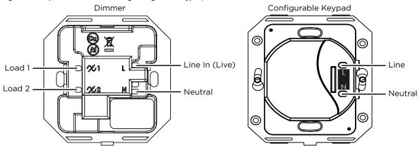
Figure 5: Multiple device locations using Configurable Keypad, without neutral connection at dimmer Configurable Keypad 0 Line In (Live) Load 1 8 Load 2 ·
