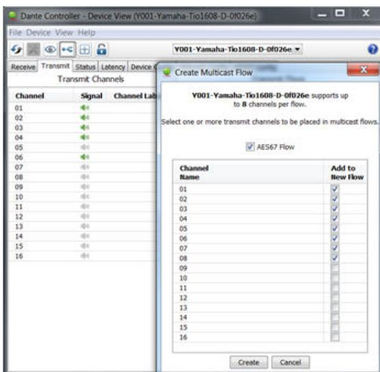
A multicast flow is now listed in the **Transmit Flows** pane of the **Transmit window**. This specifies that audio received on analog channel 1 from the cinema sound processor is routed out of digital channel 1 of the Yamaha device, channel 2 is routed out of digital channel 2, and so on. You have now completed the AES67 setup in the Dante Controller software.
