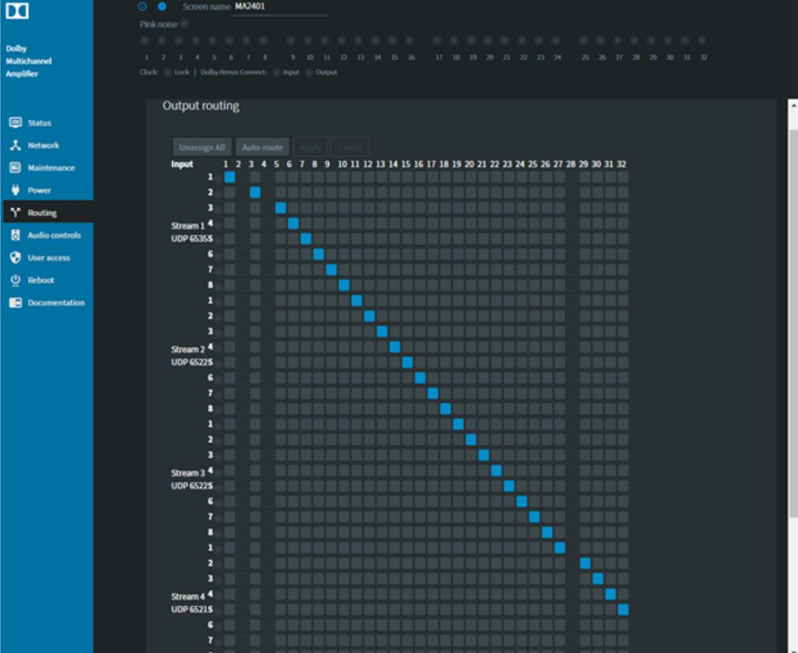
The screenshot shows the 'Output routing' screen for a Dolby Multichannel Amplifier. The interface includes a navigation bar on the left with options like Status, Network, Maintenance, Power, Routing (selected), Audio controls, User access, Reboot, and Documentation. The main area displays a grid for routing assignments. The columns represent 32 speaker outputs, and the rows represent input streams and their UDP ports. Blue squares indicate the current routing configuration.
