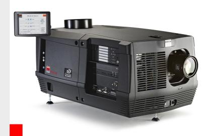
The Barco DP2K-20C is a compact digital cinema projector for theaters with screens up to 20m (65ft) wide, based on Texas Instruments' proven **0.98" DLP Cinema® chip.** It ensures a first-class movie experience with consistent picture brightness, rich contrast and vibrant colors. What's more, the DP2K-20C comes in a budget-friendly, compact form factor.
