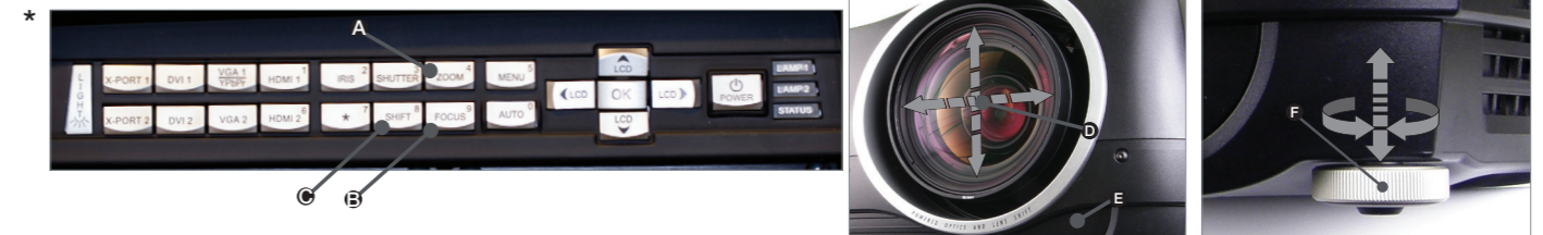
A: Zoom B: Focus C: Shift Press to activate. Adjust with arrow keys.
