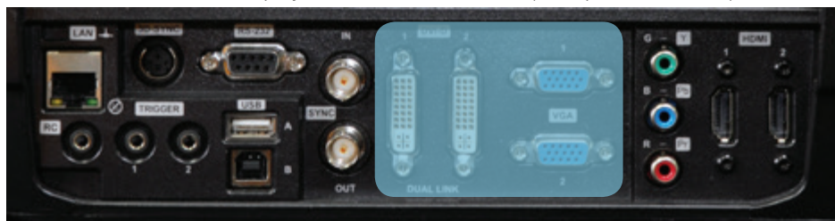
Figure 5-5. Connecting a computer source
