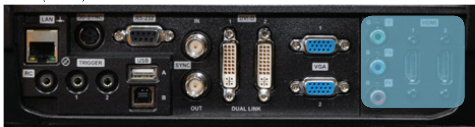
Figure 5-4. Connecting a video source
