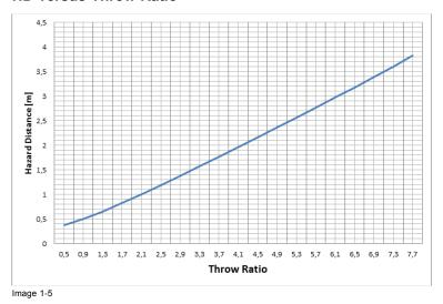
Graph shows Hazard Distance in meters versus Throw ratio of the lens
