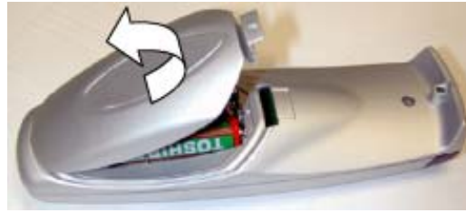
Image 2-5 Battery cover removal
