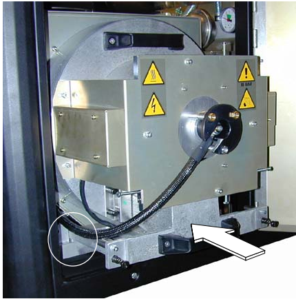
Image 7-4 Securing the lamp unit
