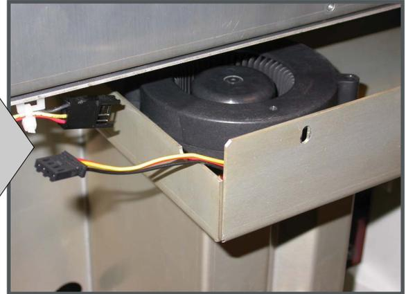
4. Replace the fan inside the fan cover and fasten the fan cover with the screws D & E as illustrated.
