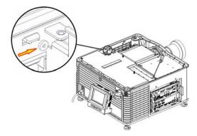
4. Push the clips on the inside, top of the service panel down and out to remove the service panel.
