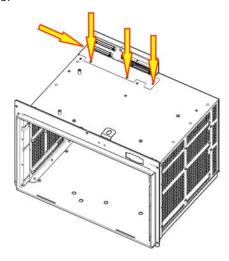
9. Disconnect the marriage interlock switch (P12) connector from the backplane.
