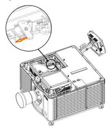
7. Pull the ejectors on the ICP outward.
