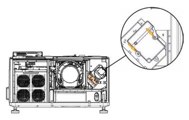
When reinstalling the light sensor module, recalibrate the footLambert (fL) readings for minimum and maximum power. See the CP2215 User manual.
