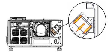
7. Slide the aperture plate out along the slotted tracks inside the IOS.
