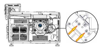
d. Rotate the yellow notch filter with the handle until you reach the correct angle. Tighten the adjustment screws when the adjustment is complete.
