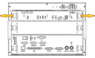
8. Pull the ICP outward out of the card cage.
