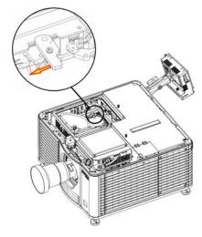
8. Remove the 5 screws that secure the card cage.
