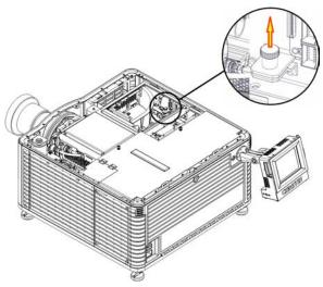
11. Tilt the card cage up and out to remove it.
