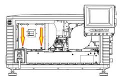
6. Remove the screw securing the anode wire. It is recommended that you use a 5 mm magnetized ball driver.
