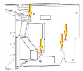
8. For the cathode blower, remove the 4 screws holding the bracket plate and duct.
