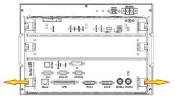
7. Pull the PIB outward out of the card cage.
