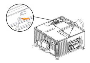
3. Open the integrator rod access door and loosen the second service panel screw.
