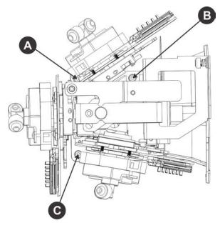
When loosening screw A, make sure you do not contact the capacitor with the hex key. If you damage the capacitor, the light engine must be returned to Christie.
