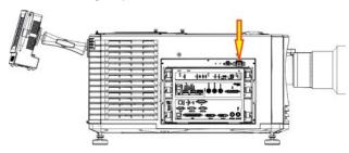
10. Pull up the release screw on the top of the card cage and then slide the card cage out along the guides.
