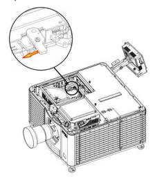
6. Pull the ejectors on the PIB outward.
