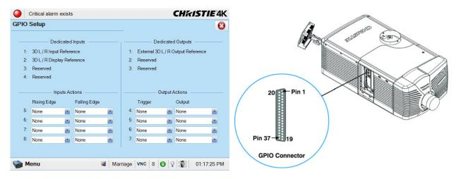
As shown below, each available pairing of pins (+/-) is defined as either an *input* or *output*. Four inputs and three outputs have already been predefined. Configure a pin as an input if you want the cinema projector to respond to an incoming signal, or as an output if you want an external device to respond to the cinema projector.
