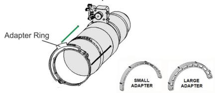
5. Verify that there is full travel of the gear ring, and the alignment of the sensor is correct.
