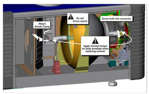
Figure 7-2 Installing the Lamp
