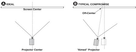
**NOTE**: Keep the cinema projector lens as parallel to the screen as possible, even if significantly above the screen center. When a particularly short throw distance combines with a very wide screen, you may have to
