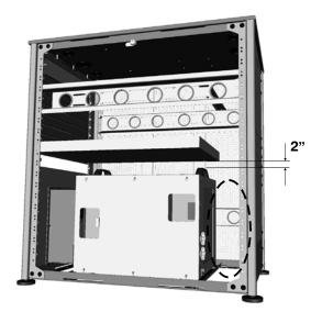
**NOTE:** *If you are using the optional rack stand, it is recommended that you use the hold down clamp (116-100101-01) in addition to the rear safety strap to firmly secure the rear feet of the cinema projector.*
