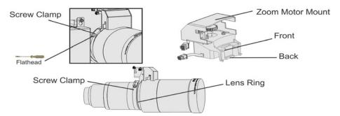
3. Remove the cover from the zoom motor mount. Keep the hardware and cover.
