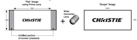
Figure 5-4 Using Wide Converter Lens to Achieve "Scope" with No Resizing
