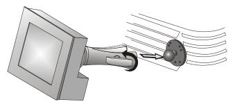
2. Tighten the mounting arm until it fits tightly on the joint.
