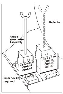
Figure 8-3 Lamp Yoke Position
