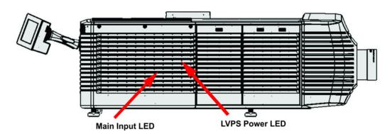
Figure 8-2 View Power Status LEDs
