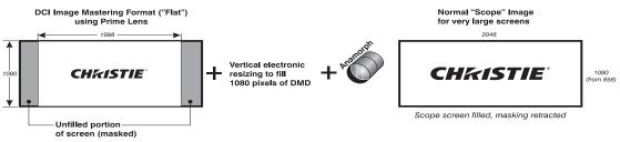
Figure 5-3 Using Anamorphic Lens to Achieve "Scope" for Large Screens
