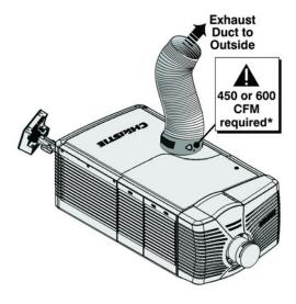
• At minimum, a 10" long, strong metal duct must be installed at the cinema projector to prevent glass shards from exiting the duct in the event of a lamp explosion.
