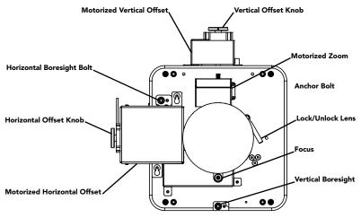
Figure 5-2 Lens Mount Components
