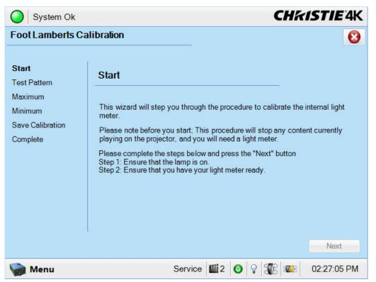
Figure 6-36 Administrator Setup: Foot Lamberts Calibration Start Window
