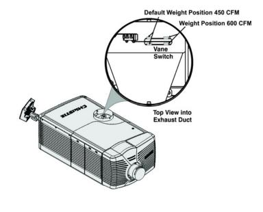
Add an extractor or a booster if there is insufficient airflow. Do not mount the extractor on the cinema projector as this may introduce some vibration into the image. **NOTE:** *To prevent the cinema projector from overheating or becoming unsafe, an alarm sounds if the duct is obstructed or a fan fails. It is recommended that you regularly verify that the exhaust is functioning correctly.*
