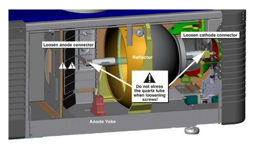
Figure 7-1 Removing the Lamp
