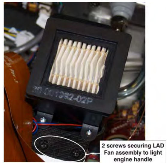
Figure 5-16 Remove LAD Fan Assembly
