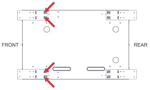
3. Install four M5 screws for each rear plate and torque the screws.
