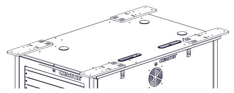
2. Install two M5 screws for each front plate and keep the screws loose.
