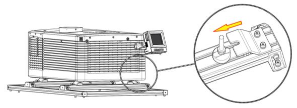
5. Tighten the 2 screws on each of the 4 foot brackets.
