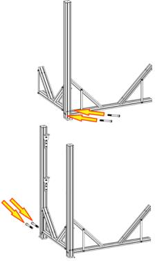
4. Attach the left rear post to the other side of the side brace from step 1 with 2 M12 x 100 mm bolts.
