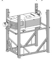
Make sure that all 4 brackets are supporting the shelf, and that the supporting surfaces of the brackets are flush with the bottom of the shelf.
