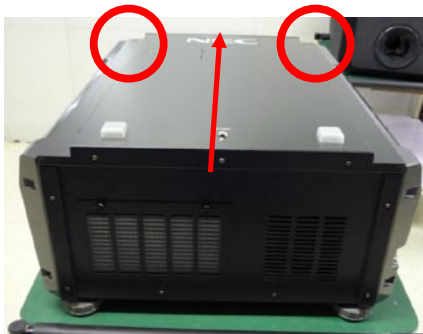
Loosen 2 screws on the top cover. Torque: 7~8 kgf-cm.
