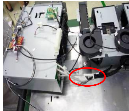
Unplug the 2 pcs lamps and ballasts cables to take power module off.
