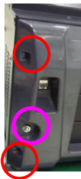
Use key to unlock the screw and open the left outside cover. Torque: 7~8 kgf-cm.
