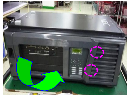
Loosen 2 screws and open and take out 2 pcs left outside cover.
