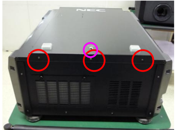
Use key to unlock the screw and open the top cover. Then, loosen 3 screws on the top cover. Torque: 7~8 kgf-cm.
