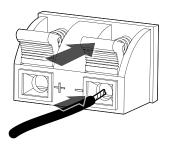
6 To keep polarity correct, connect the amplifier's + (positive) channel to speaker's + (positive) channel and the amplifier's - (negative) channel to the speaker's - (negative) channel. To avoid shorts, keep stray strands clear of adjoining connectors.
