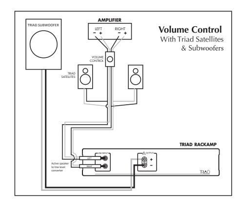
From the volume control, "Y" the speaker wires so that one set goes to the satellites, and the other set goes to the Triad Subwoofer RackAmp through active speaker to line level converters.
