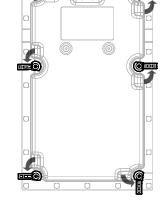
Mounting doglegs will move outward and tighten to secure the speaker to the drywall.
