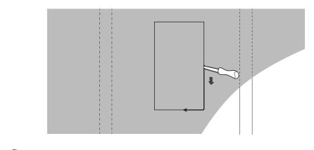
Pull pre-wired speaker cable through the cutout or run the speaker 4 wire from the cutout to the amplifier location.
