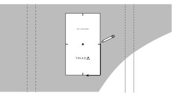
Slowly cut along the outlined mark with a drywall knife/saw, trying not to chip out the drywall excessively.
