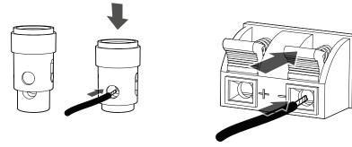
To keep polarity correct, connect the amplifier's + (positive) channel to speaker's + (positive) channel and the amplifier's - (negative) channel to the speaker's - (negative) channel. To avoid shorts, keep stray strands clear of adjoining connectors.
