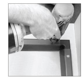
B Drill pilot holes into cabinet base for (8) #10 x 1-1/2" Pan Head Phillips Screws.
