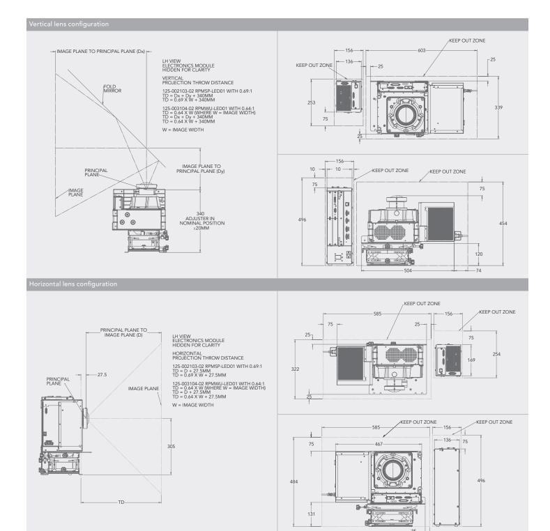
Notes: A. Dimensions are millimeters B. Adjuster is in neutral position C. Stay out zone required for air flow, adjuster range, cable routing and service D. Projection distance tolerance  $\pm$  1.5% E. The electronics module is shown in nominal position relative to projector's body it can be relocated to the left up to 50, and  $\pm$  20mm back and forth from nominal position
