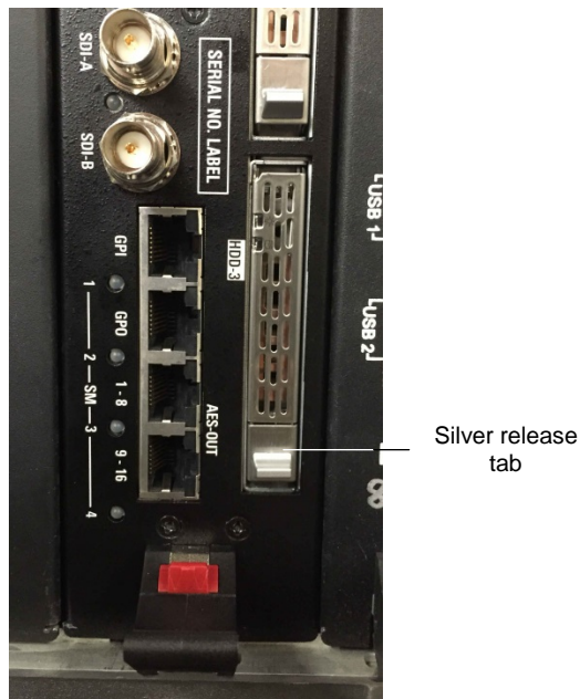
Figure 7-6 Silver Latch on Hard-Disk Drive
