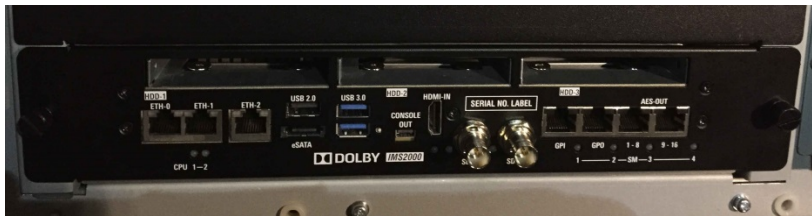
Figure 5-8 IMS2000 Inserted Without Hard-Disk Drives
