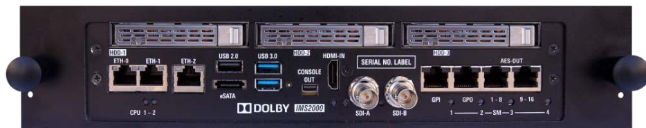
Figure 4-2 IMS2000: Front View
