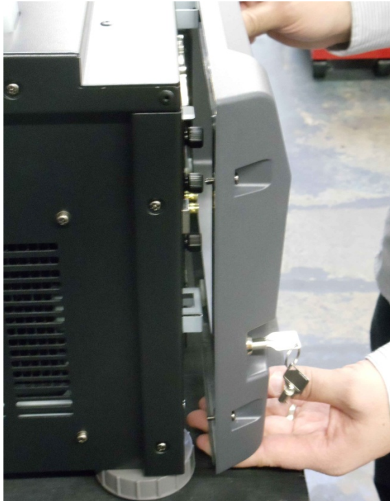
Figure 5-13 Reattaching the Projector Cover
