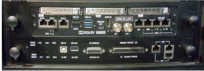
Figure 6-7 Hard-Disk Drives Inserted
