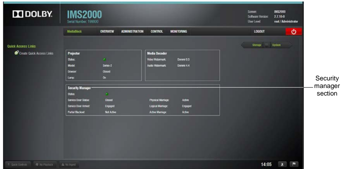
Figure 5-36 Security Manager Section
