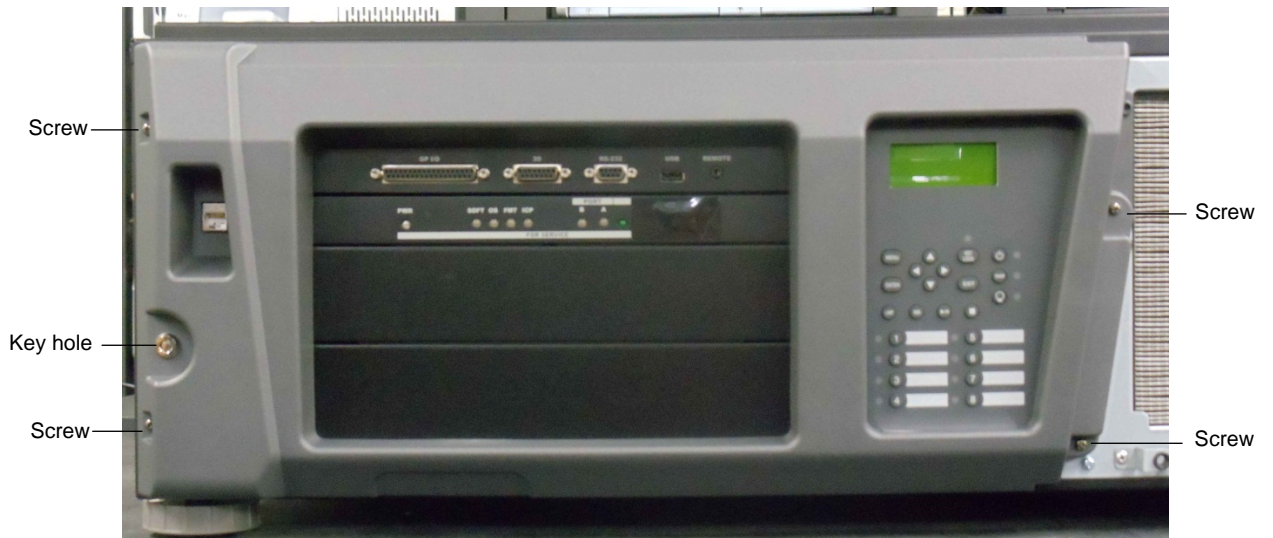
Figure 5-3 Removing Filter Screws
