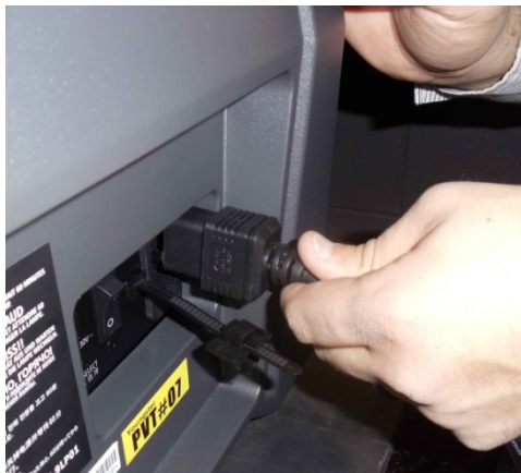
Figure 5-21 Connecting the Power Cable
