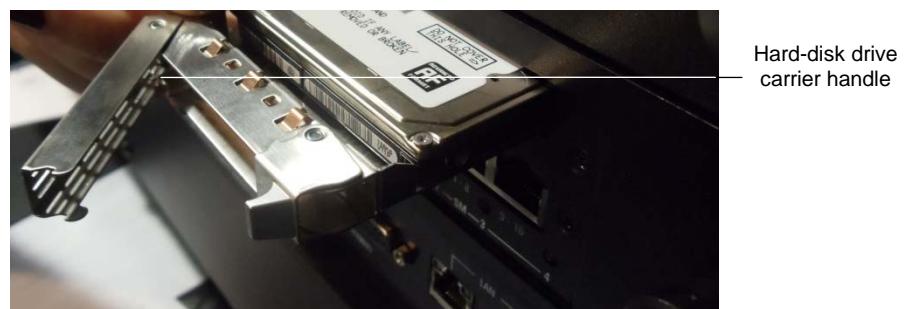
Figure 6-6 Inserting Hard-Disk Drive
