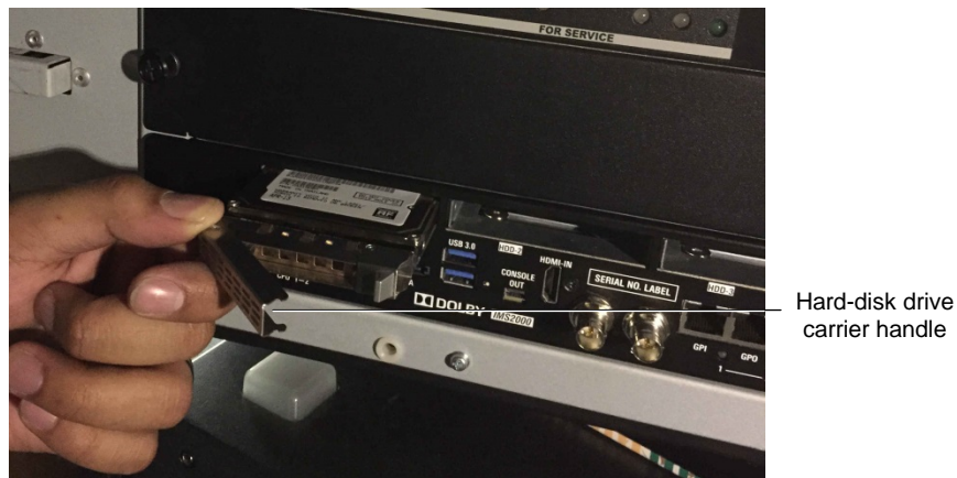
Figure 5-11 Hard-Disk Drive Latch
