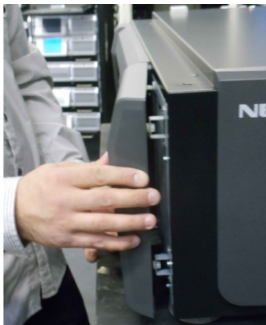
Figure 5-15 Reattaching the Filter Cover
