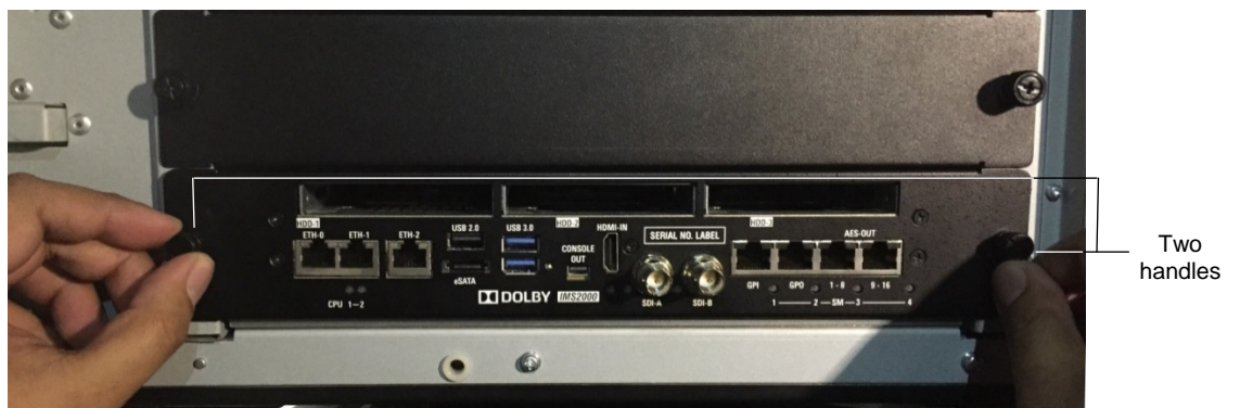
Figure 5-9 Securing the Board
