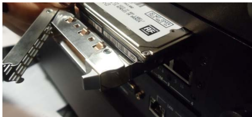
Figure 16-1 Hard-Disk Drive Removal
