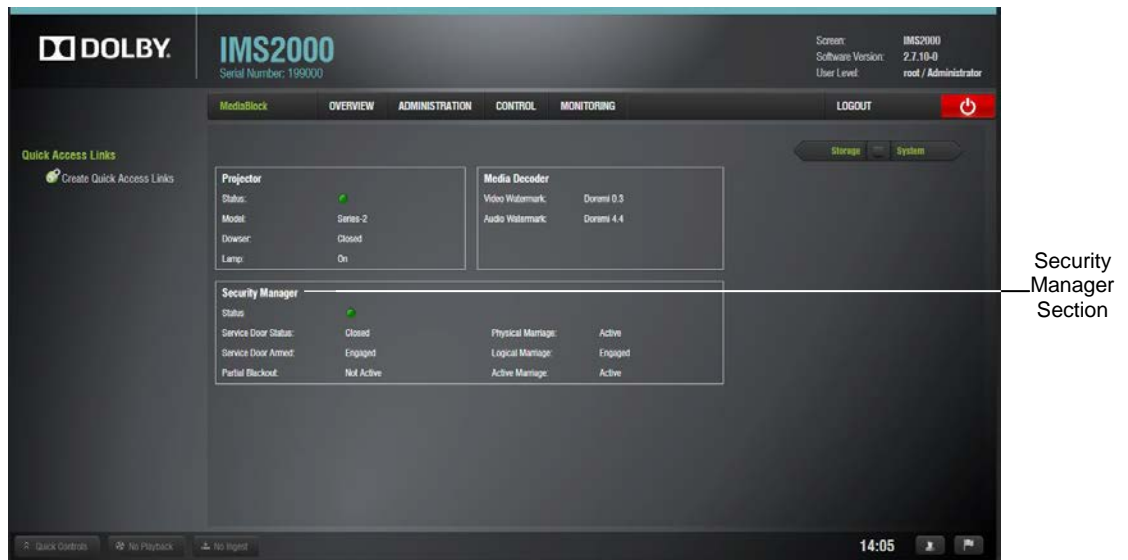
Figure 6-19 Security Manager Section
