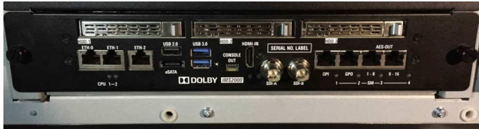
Figure 5-12 Hard-Disk Drives Inserted
