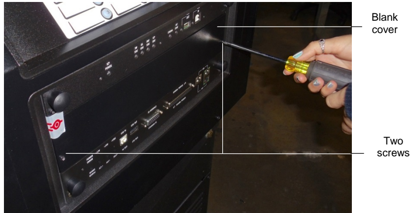
Figure 6-2 Unscrewing Blank Cover
