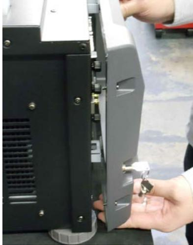
**Figure 5-7** Replacing the projector cover
