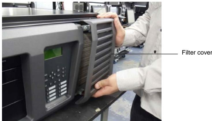
**Figure 5-1** Removing the projector filter
