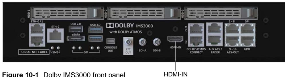
Figure 10-1 Dolby IMS3000 front panel
