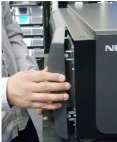
**Figure 5-9** Replacing the filter cover
