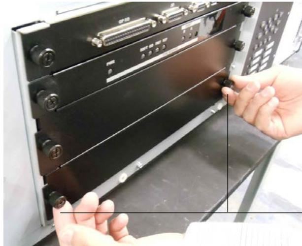
**Figure 5-5** Removing the slot cover
