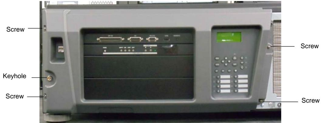
**Figure 5-2** Removing filter screws
