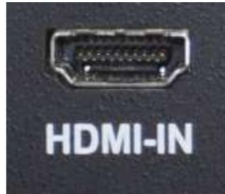
Figure 36: HDMI-In Connector
