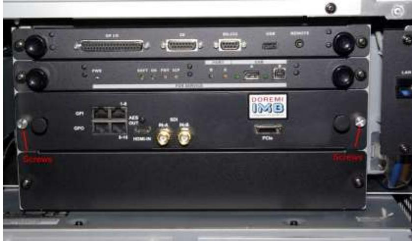
**Figure 10: IMB Installation**
