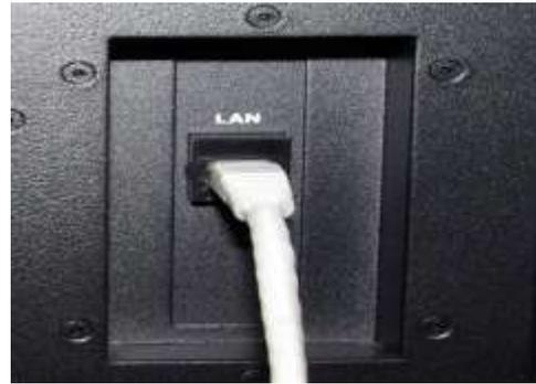
**Figure 12: Ethernet Cables**
