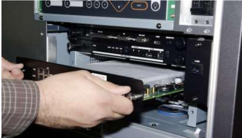
**Figure 9: IMB Installation**
