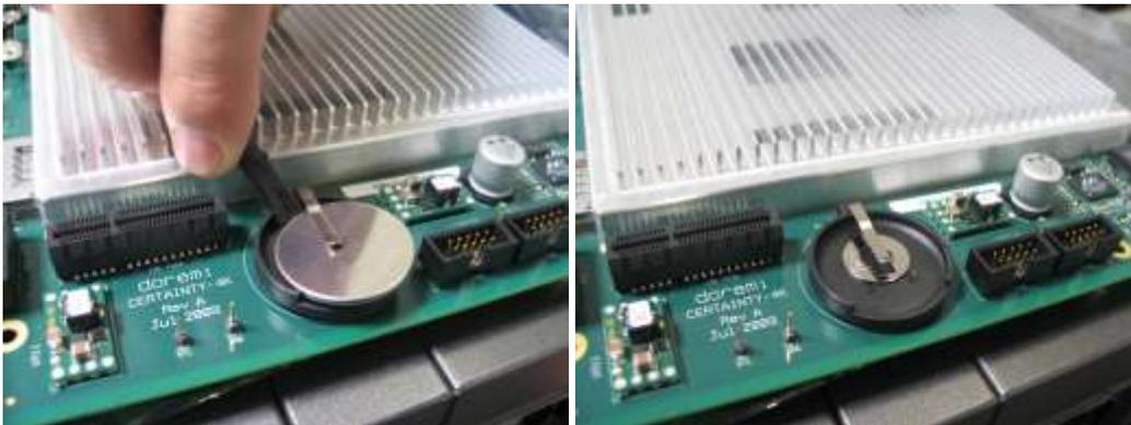
**Figure 40: IMB Battery Removal**
