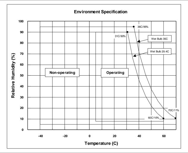
Figure 4 Limits of temperature and humidity
