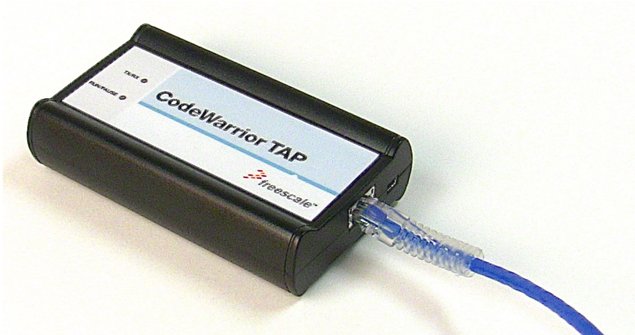
Figure 4. CodeWarrior TAP probe with an RJ45 cable attached
