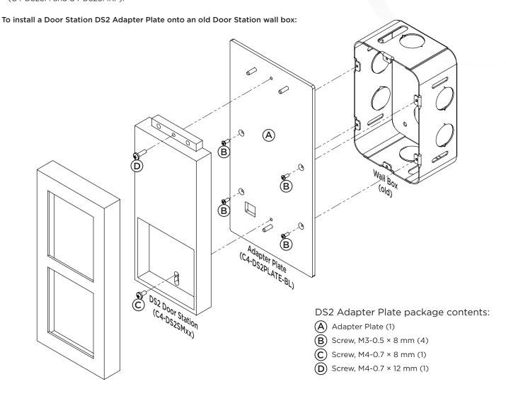
**Tip:** For a more water-resistant and draft-resistant mounting surface, fill the existing (old) wall box with expanding insulation foam, then trim it flush with the wall after curing. You can also use waterproof caulk or sealant between the adapter plate and the wall surrounding the old wall box.
