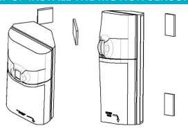
Install the Motion Sensor on a clean surface using the 2-sided tape provided. It can be installed on a flat surface or in a corner, vertically, horizontally or upside down.
